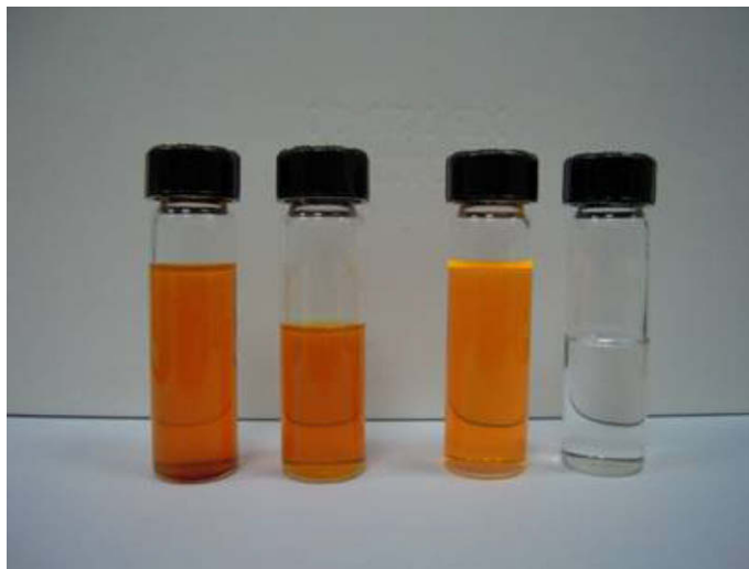
Fig. 1. The comparison of oxygen resistances for 2CT and rubrene in chloroform solution. (from left to right, the first and the third samples are initial 2CT and rubrene solution; the second is 2CT solution after three months and the fourth is rubrene solution after three days, respectively).
